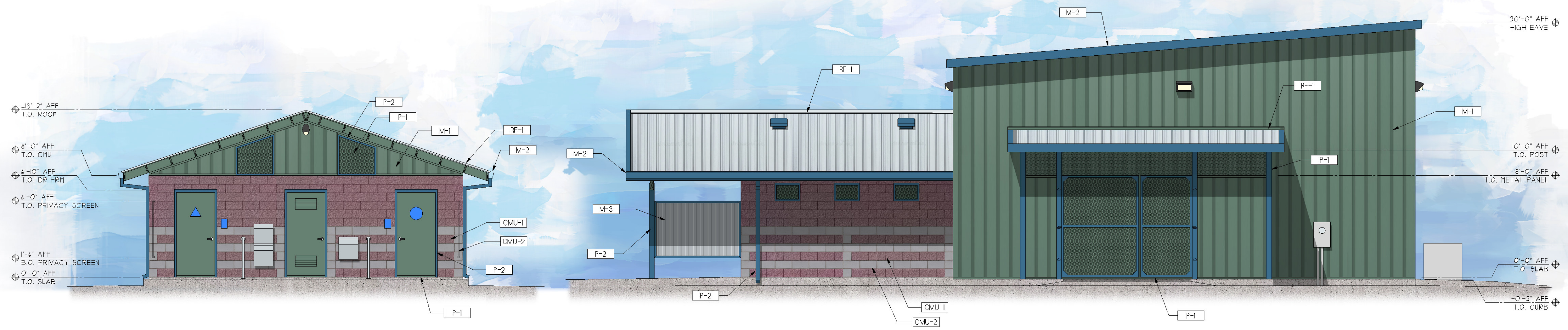
2 NORTH ELEVATION AT RESTROOM FRONT WALL SCALE: 1/4"=1'-0"
